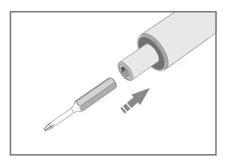
1. Put the bit out from the storage case and into the rotary axis.
