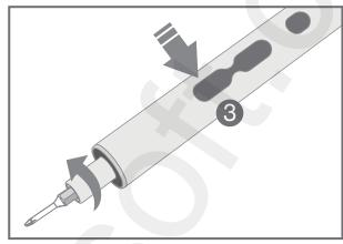
2. Press 3, tighten or screw the screws.
