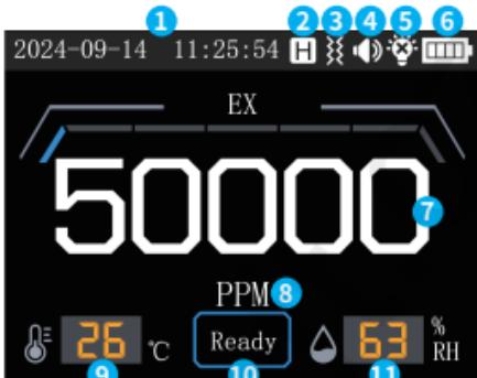
④**Buzzer alarm:** Indicates whether the alarm function is enabled
